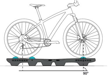
Measure (H) the distance between the centre of the wheels of the bicycle to be use on GH-565-1.
